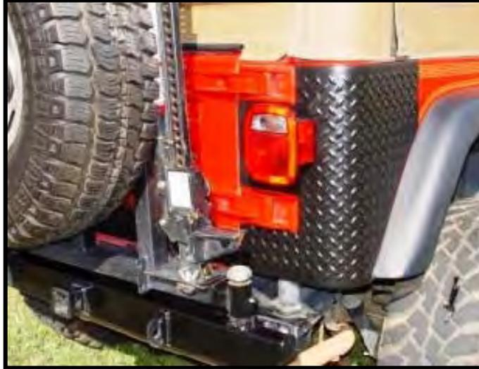
**Step 1:** Remove both left and right side rear taillight assemblies. This will require the removal of 3 bolts for each light that are assessable from the inside of the tail light assembly and from the upper inside of the fender. The lower plastic fender cover can be pulled back without removing. The left side license plate holder and fuel filler neck will also be removed.
